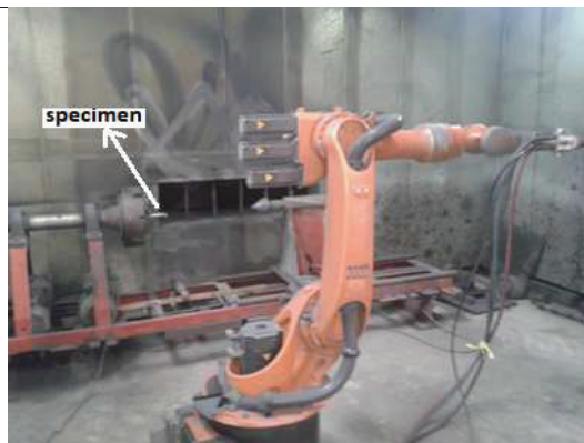
Fig 3.7: Experimental setup for HVOF coating process
