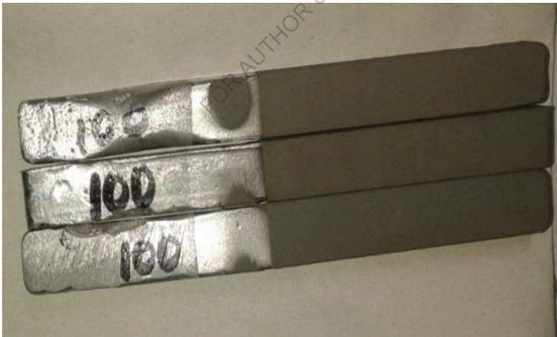
Fig 6.5: WC-Co coated Al/2%RHA composites
